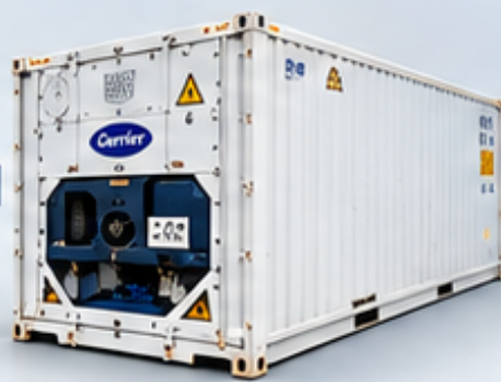
Reefer Container For temperature-controlled cargo
